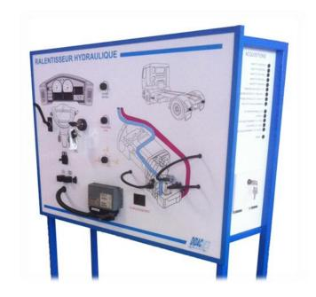
The hydraulic retarder is a braking system located on the propeler shaft (gear boxes output). The vehicle kinetic energy is converted in hydraulic then calorific energy into a temperature exchanger. Many technical and economic advantages done of this type of retarder are a device very used by Trucks manufacturers.
