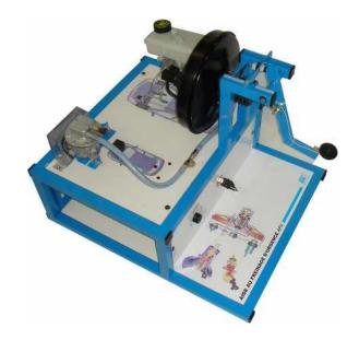
This pedagogic unit allows a complete study of the AFU system associated with ESP and with the distance regulator.
