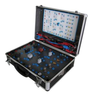
The electric's notions became inescapable in the automotive maintenance sector. A good understanding of these physical phenomena is fundamental to identify the functioning of a system and realize a relevant diagnosis. DIDAC BDH realized a suitcase "all inclusive" which allows to analyze electric basic assemblies from components most usually used.
