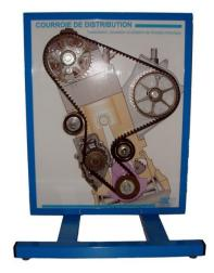
The timing belt links the crankshaft to the camshaft through the coolant pump and the injection pump. The path of the belt is determined by the position of the gears and rollers.
