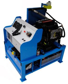
The proposed engine bench is a new technology which allows the manufacturer to comply with the EURO 4 and EURO 5 norms. It is equipped with an injection system (*common rail type*) and with an urea injection system with a catalyst. This modern unit allows to study, in addition to the injection system, a very large range of motorization aspects (load circuit, starting circuit, oversupply, cooling, lubrication, fixing...)
