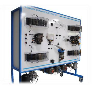
The electronic braking system EBS is a new system already in use at many truck manufacturers (RENAULT TRUCK, SCANIA, MERCEDES, VOLVO). This system includes the ABS and ASR features? AND OPTIMISE THE BRALING EFFICIENCY This is a little technologic revolution!
