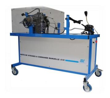
This teaching kit is used to study gearboxes both from the functional (adaptation to the engine and the vehicle, calculation of ratios, study of synchronization) and structural perspectives (drivetrain, design, rotation guides, sealing, etc.).
