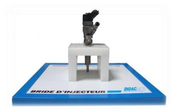
The high-pressure injection systems used on diesel engines have seen the introduction of electrically controlled injectors. Due to the central position of the control coil, the high-pressure coupling is located on the side. This means that the injectors can no longer be screwed into the cylinder head and that each injector is secured by a clamp.
