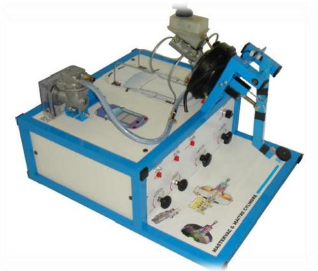
This pedagogic unit allows a complete study of the braking assistance device (mastervac) and of the master-cylinder.
