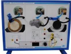
A blue metal cabinet containing rotation speed sensors, including inductive sensors for ABS-EBS and magneto-resistive sensors for ABS, along with a hall effect sensor for vehicle speed, with associated wiring and connectors. |
