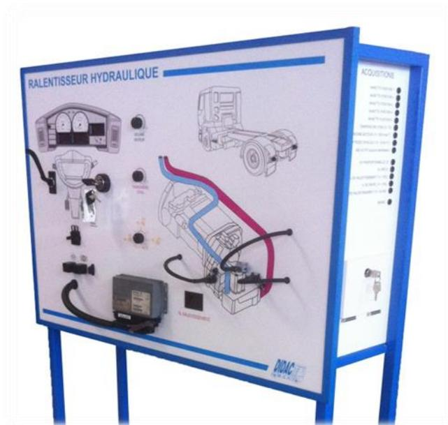
The hydraulic retarder is a braking system located on the propeller shaft (gear boxes output). The vehicle kinetic energy is converted in hydraulic then calorific energy into a temperature exchanger. Many technical and economic advantages done of this type of retarder are a device very used by Trucks manufacturers.
