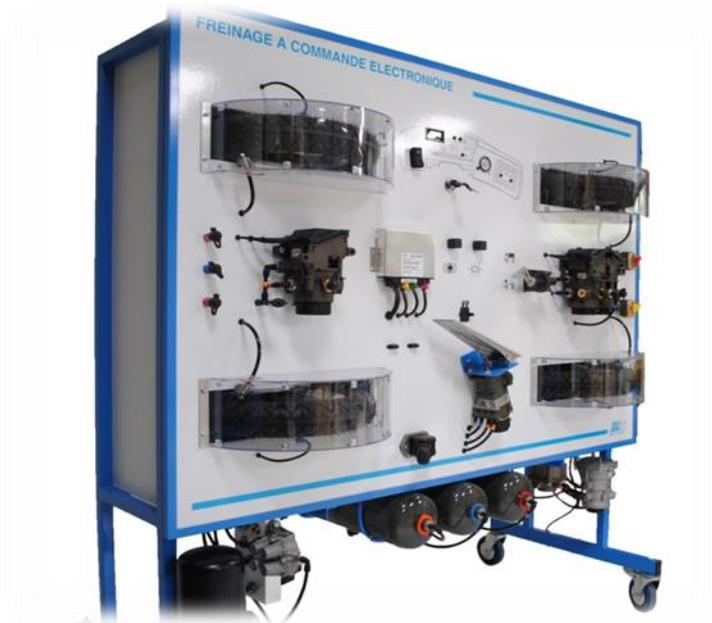
The electronic braking system EBS is a new system already in use at many truck manufacturers (RENAULT TRUCK, SCANIA, MERCEDES, VOLVO). This system includes the ABS and ASR features? AND OPTIMISE THE BRAKING EFFICIENCY
