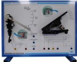
A blue metal cabinet containing position sensors, including an angular potentiometer for the accelerator pedal and an inductive sensor for the under-body height, with associated wiring and connectors.                           |
