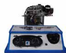
The dashboard with the controls and indicators associated with the semiautomatic gearbox
