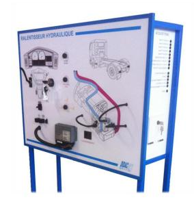
The hydraulic retarder is a braking system located on the propeler shaft (gear boxes output). The vehicle kinetic energy is converted in hydraulic then calorific energy into a temperature exchanger. Many technical and economic advantages done of this type of retarder are a device very used by Trucks manufacturers.
