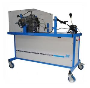
This teaching kit is used to study gearboxes both from the functional (adaptation to the engine and the vehicle, calculation of ratios, study of synchronization) and structural perspectives (drivetrain, design, rotation guides, sealing, etc.).
