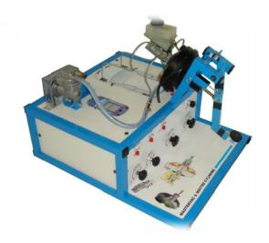
This pedagogic unit allows a complete study of the braking assistance device (mastervac) and of the master-cylinder. It is specially appropriated for functional and structural analyze lessons, mechanics, technology and exercises. It can be used from BEP to BTS (French National Education).
